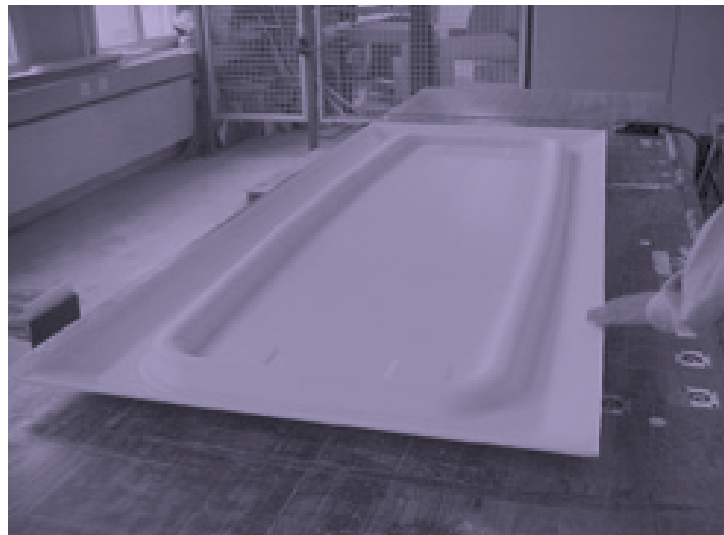
THE GROOVE IN THE BOTTOM LAYER OF THE TABLE PROVIDES STRUCTURAL
