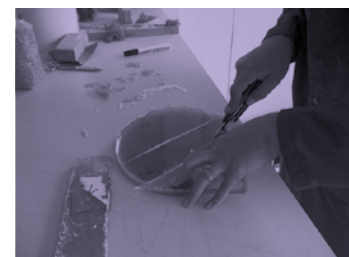
CUTTING MATERIAL SAMPLES THAT WILL BE SUBJECTED TO A BREAK TEST.
